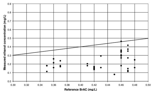
Fig 5. The ethanol concentration measured with the breath analyzer prototype in subjects who simulated sleeping, in relation to the breath alcohol concentration measured during vital capacity expiration with a reference instrument (Alco-Sensor FST, Intoximeter INC, U.S.).
