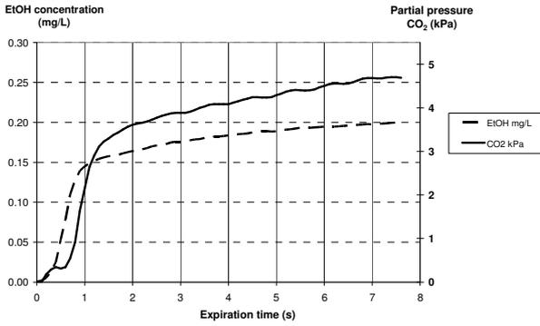
Fig. 1 Expirogram for ethanol and CO<sub>2</sub> recorded by a modified evidential breath analyzer (Evidenzer, Nanopuls AB, Sweden).
