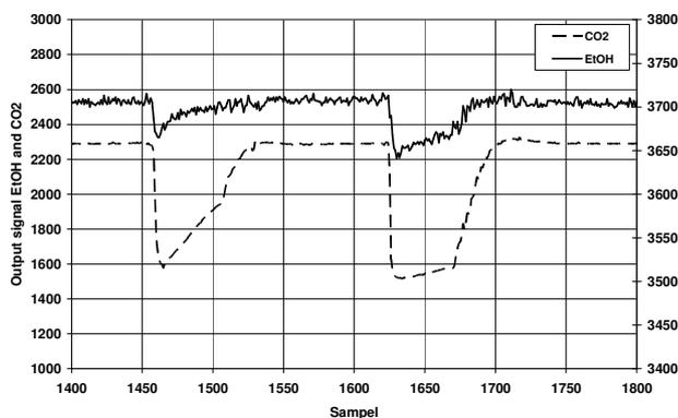
Fig 3. Decrease of the two output signals due to the concentration of ethanol and  $\text{CO}_2$  in expired air. The figure also illustrates the two channels correlation in signal level. The ethanol signal has a linear response to increased concentration, whereas the  $\text{CO}_2$  signal has a logarithmic response. Vertical scale is A/D bits (0.105  $\mu\text{V}/\text{bit}$ )
