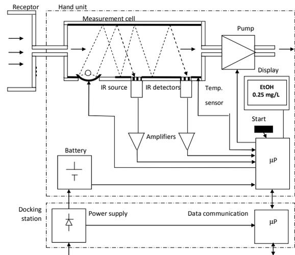
Fig. 2 Schematics of the outline of the breath analyzer.
