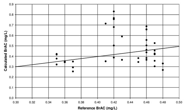
Fig 6. The breath alcohol concentration (BrAC) compensated for the sample dilution (the  $\text{EtOH}/\text{CO}_2$  ratio times 3.9 kPa) plotted against the BrAC measured with the reference instrument (Alco-Sensor FST, Intoximeter INC, U.S.). The residual standard deviation was 0.15 mg/L.
