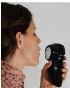
Figure 2. A prototype of the handheld breath alcohol analyser designed for directed breath.
